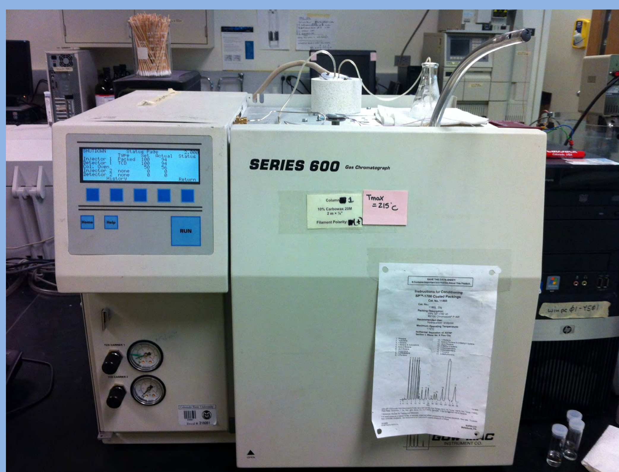
Figure 2. Gow-Mac Series 600 GC equipped with a Thermal Conductivity Detector (TCD).
