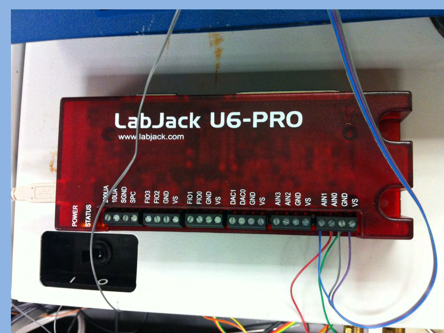
Figure 3. LabJack U6 Multi-Channel Analog to Digital Converter (ADC).
