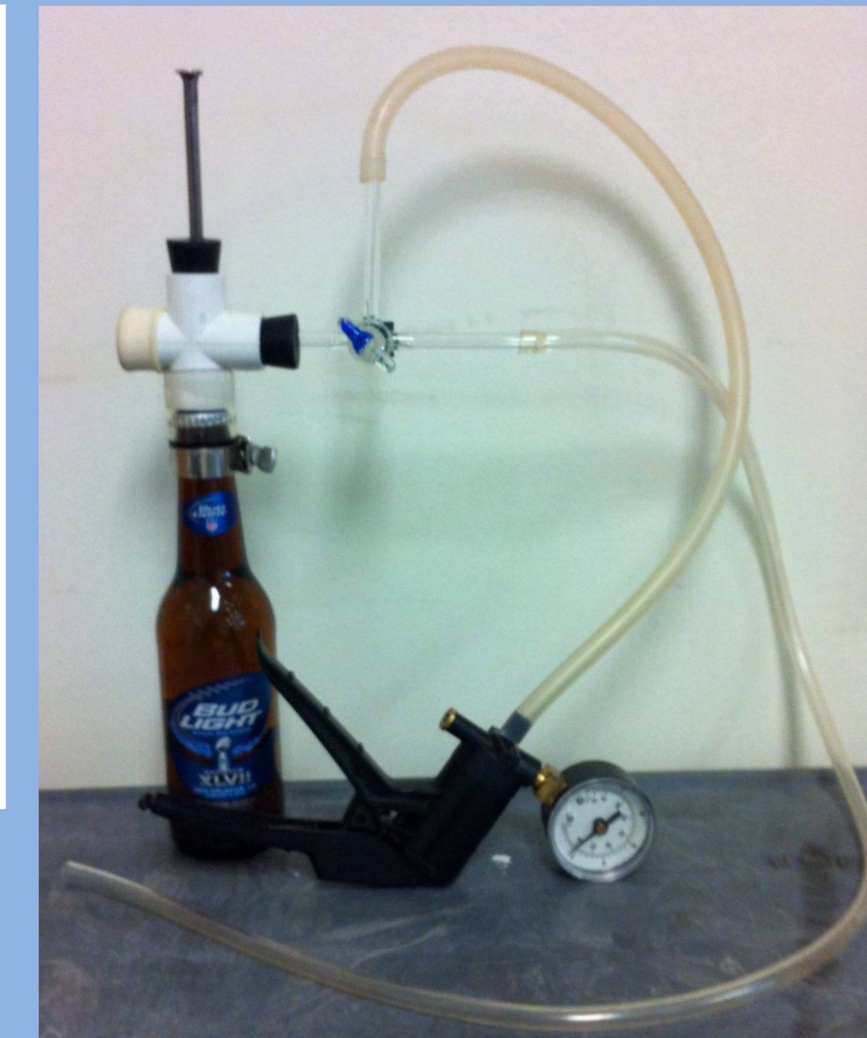
Figure 4. Headspace apparatus composed of common laboratory equipment.
