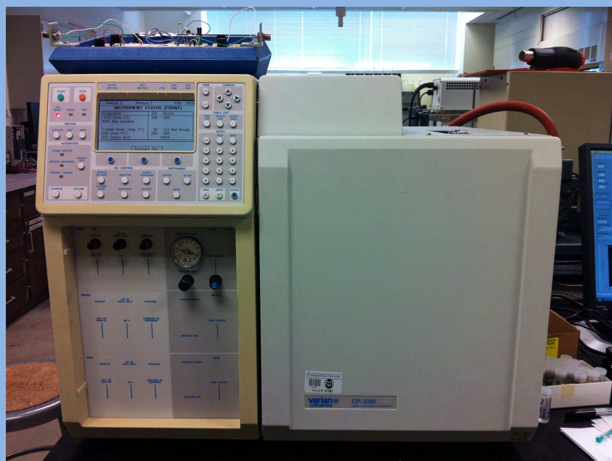
Figure 1. Varian CP 3800 GC equipped with a Flame Ionization Detector (FID).
