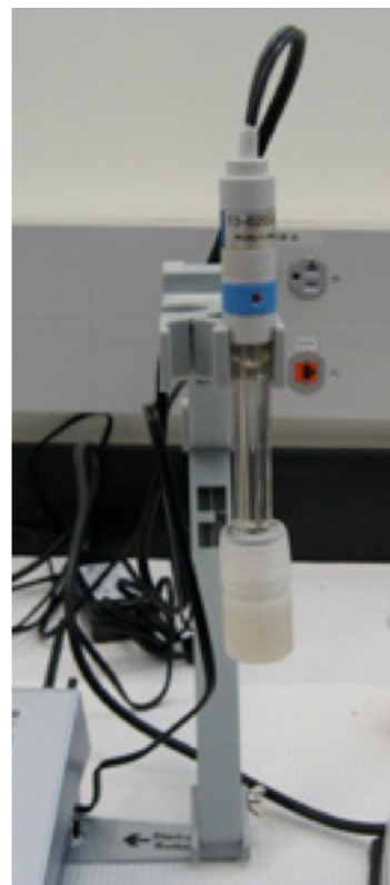
Figure 1. pH combination probe suspended in electrode arm with storage vial covering the active tip.
