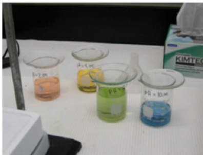
Figure 2. Standard buffer solutions used for calibration of the pH meter. Color-coded acid-base indicators are added in the solutions to provide convenient visual identification of the solutions.
