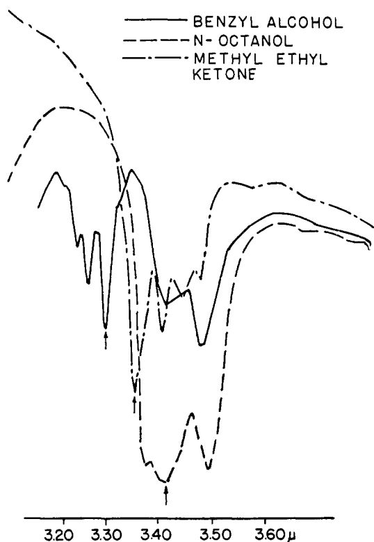
Figure 6. Infrared Absorption Structure in C-H Region for Benzyl Alcohol, n -Octanol, and Methyl Ethyl Ketone
