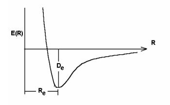
Figure 6.1. The effective internuclear potential as a function of internuclear separation.
