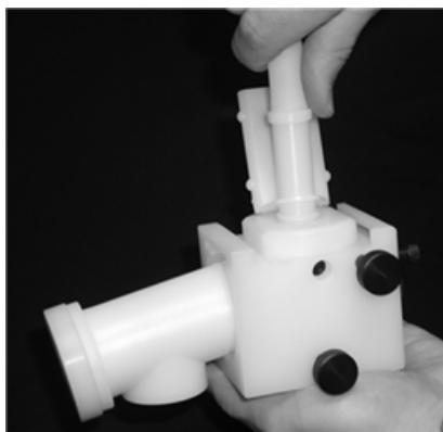
Figure 12. Screw the drain tube into the nebulizer block
