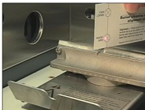
Figure 22. Aligning the burner
