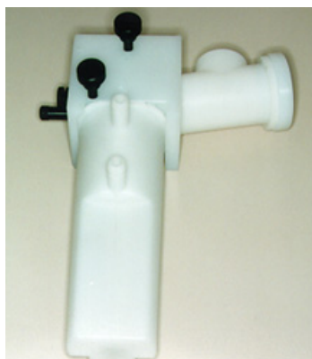
Figure 11. Complete nebulizer/spraychamber assembly
