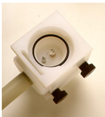
Figure 9. O-ring in place in the nebulizer block
