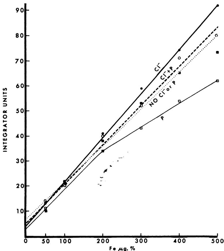
Fig. 7. Effects of chloride and phosphate on standard iron curve.
