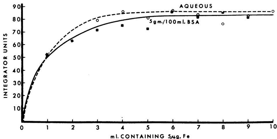
Fig. 6. Areas generated by  $5 \mu\text{g.}$  of iron in varying volumes of diluent.
