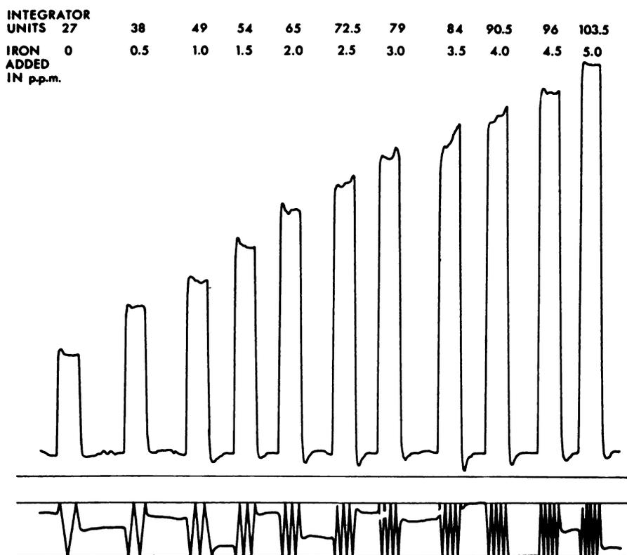
Fig. 5. Recorder curve with integrations generated by 1-ml. samples containing increasing increments of iron.
