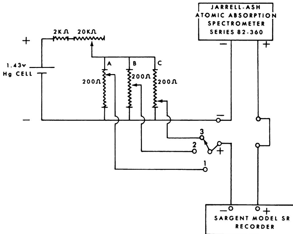
Fig. 1. Zero suppression circuit for adapting 10 mv recorder to atomic absorption spectroscopy. Variable resistances (A, B, and C) are adjusted so that bucking EMF is 5, 8, and 9 mv given a scale expansion of  $\times 2$ ,  $\times 5$ , and  $\times 10$ , respectively.
