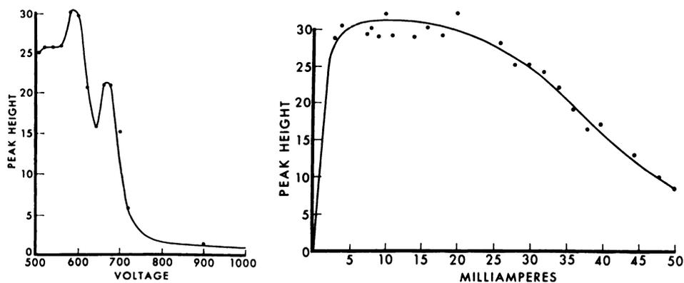
**Fig. 2** (left). Effect of varying voltage to photomultiplier tube at optimum gain. Zero adjustment was made using gain control for each determination. Milliamps to hollow cathode = 20. **Fig. 3** (right). Effect of varying current to hollow cathode lamp.
