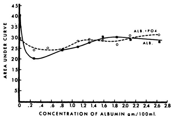
Fig. 8. Effect of increasing concentrations of albumin and phosphate on 200  $\mu$ g./100 ml. iron standard.
