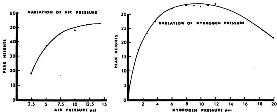
**Fig. 4.** Effect of varying hydrogen and air pressures. At left, hydrogen pressure is 8 psi. At right, air pressure is 7.0 psi.
