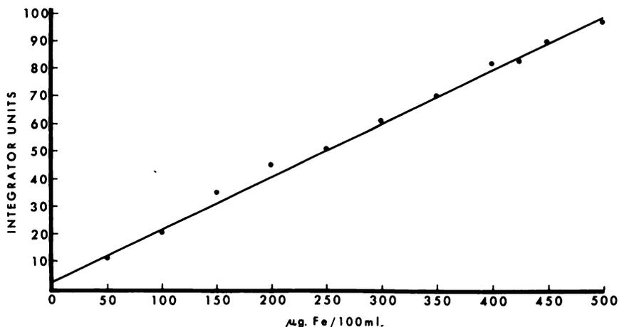
Fig. 9. Standard iron curve. Standards prepared in 6 gm./100 ml. iron-free albumin solution.
