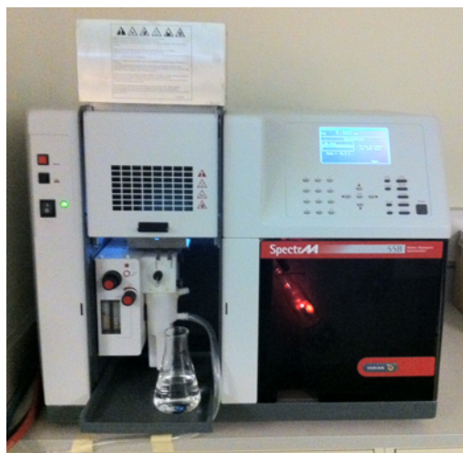
Figure 2. The Varian SpectrAA 55B atomic absorption spectrometer. The user interface and display are located at the upper right, the light source at the lower left, the sample nebulizer, aspirator and reservoir at the lower left, the burner at the upper left and the exhaust chimney at the extreme upper left.
