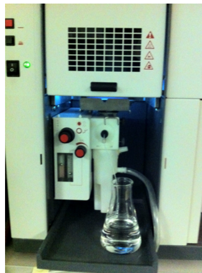
Figure 6. Detail of the sample area. The Erlenmeyer flask is the distilled water reservoir. While the flame is burning water must flow continuously into the nebulizer and the drain tube must be unobstructed.
