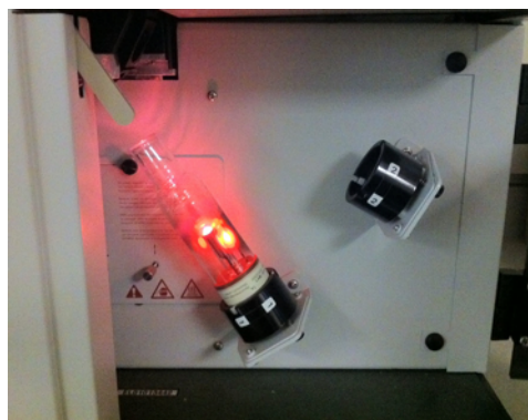
Figure 4. A hollow cathode lamp serving as a light source for absorption measurements installed in lamp position #1. Another lamp can be installed in position #2 to facilitate rapid switching between different elements.
