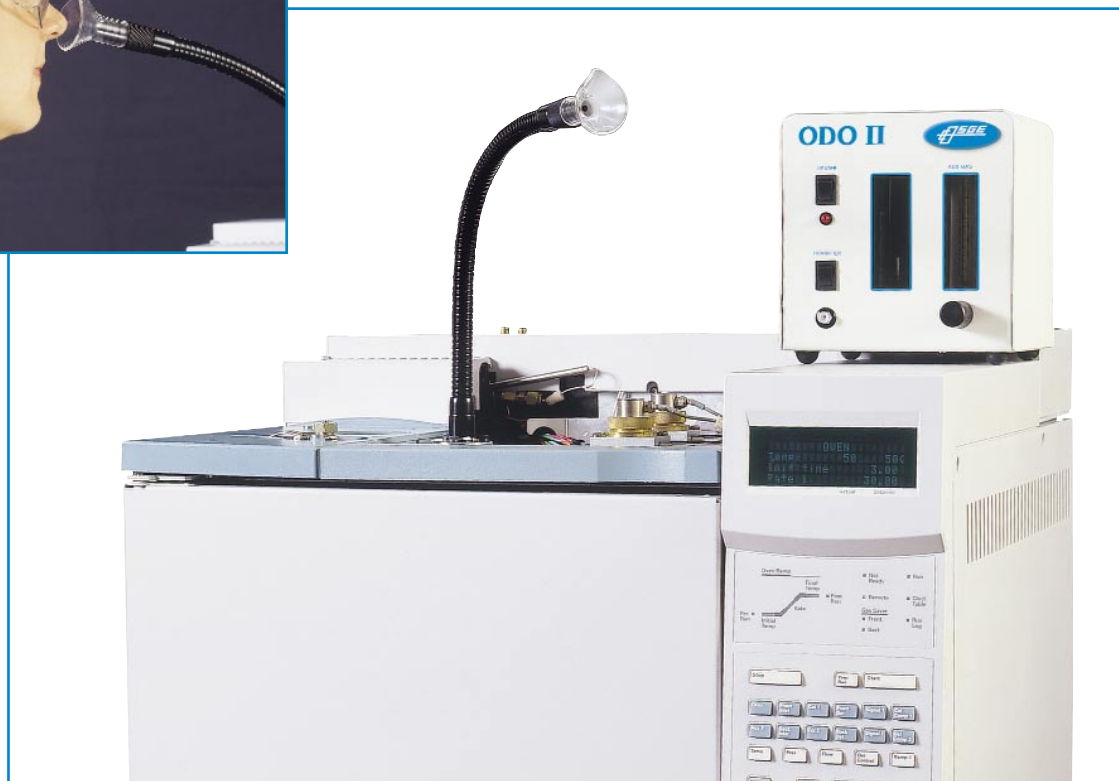
Figure 1. The new olfactory system incorporates a flexible heated transfer line for easy positioning of the nose cone away from the hot zones of the GC. This makes “sniffing” ergonomic and comfortable while ensuring each sample component is transferred to the cone without loss due to condensation or activity. The system also incorporates the control module, as shown.
