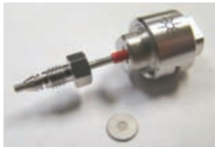
Figure 59. Inline filter for the 1290 Infinity LC, PN 5067-4638
