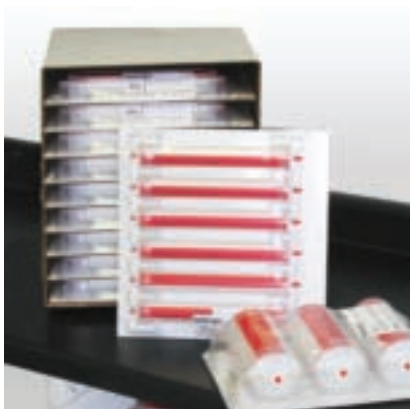
Figure 8. Flash chromatography columns: plastic columns filled with a variety of media – typically silica.
