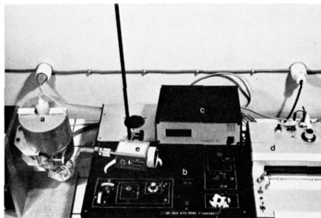
Figure 1. Comprehensive view of the apparatus; (a) microcalorimeter (b) control and calibration system (c) digital thermometer (d) recorder (e) microburet.
