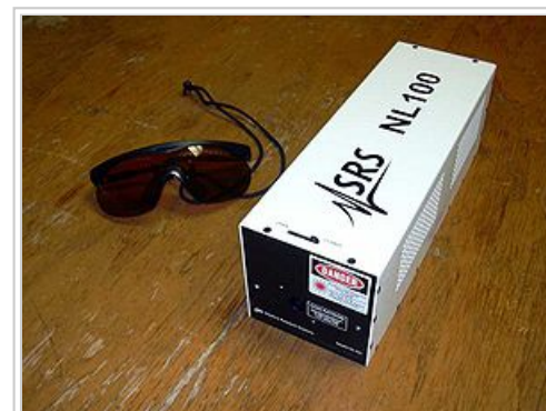
A 337nm wavelength and 170 μJ pulse energy 20 Hz cartridge nitrogen laser
