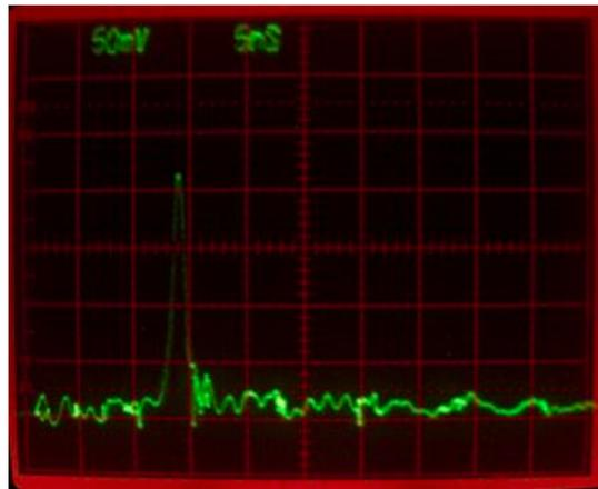
The next photo is a trace of the light from the spark gap of that same nitrogen laser. As you can see, the 0-100% risetime of the spark gap is about **18 nsec**.
