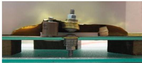
The top electrode is mounted on a broad piece of brass shim that comes off the top capacitor plate, so it avoids part of the inductance of the large one-turn coil that is inherent in Small's design. In addition, the gap has a starting capacitor across it [the small brown cylinder just to the left of the gap], which speeds it up even further. As a result, this gap is *at least* as fast as the one in the SciAm laser, and in fact it is probably significantly faster.
