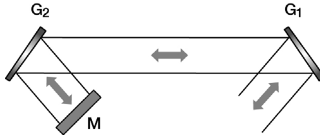
Figure 13-6. A grating-based pulse stretcher. Intermediate lenses are not shown.
