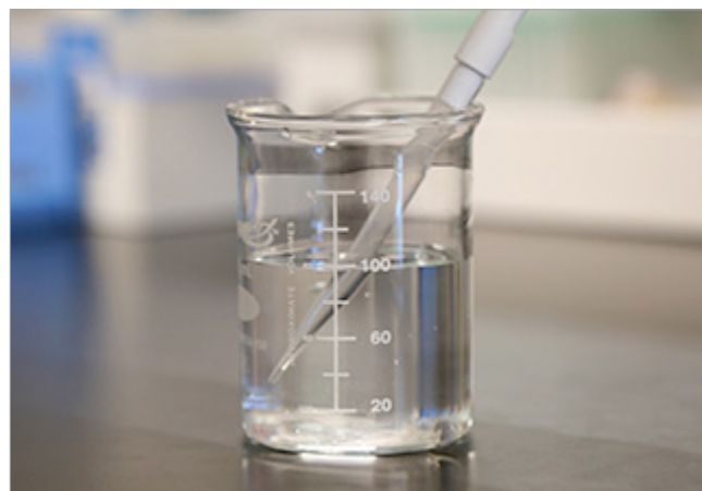
Figure 2: Minimize error by using proper pipetting technique: always hold the tip perpendicular to and just below the liquid surface. Holding it at an angle or deep under the surface can result in inaccurate volumes.
