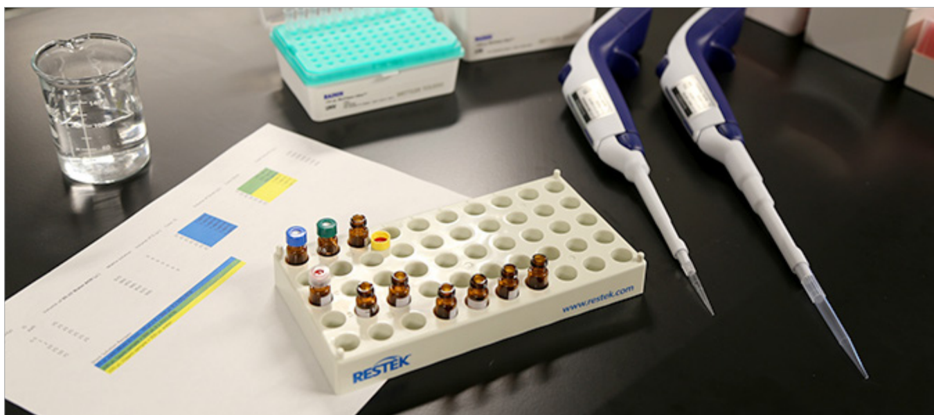
Figure 4: Using a pre-calculated, color-coded workflow for preparing calibration standard solutions and moving vials in a rack to track step completion is a simple way to prevent costly errors.
