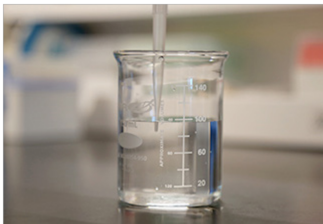
Figure 2: Minimize error by using proper pipetting technique: always hold the tip perpendicular to and just below the liquid surface. Holding it at an angle or deep under the surface can result in inaccurate volumes.
