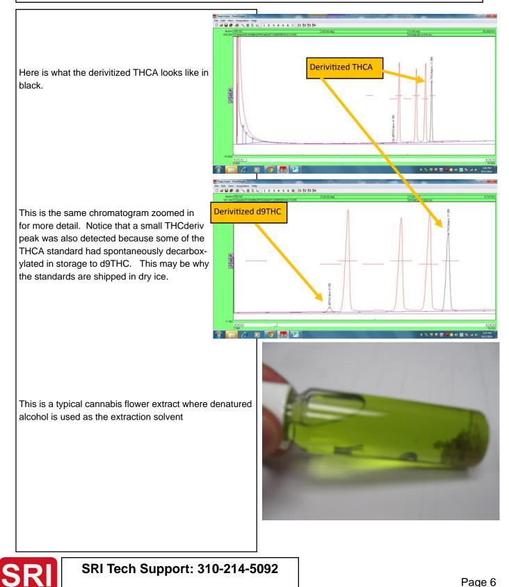
After evaporating the alcohol from 50ul of the cannabis extract you can see the residue including the green colored chlorophyll in the bottom of the 100ul insert.
