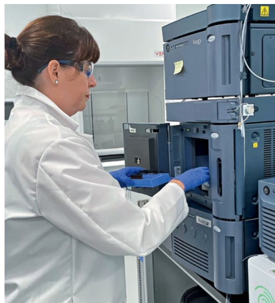
Michelle Sallin, the Maryland Cannabis Administration’s chief of laboratory services and laboratory director, optimizes a liquid chromatography method for measuring cannabinoids.
