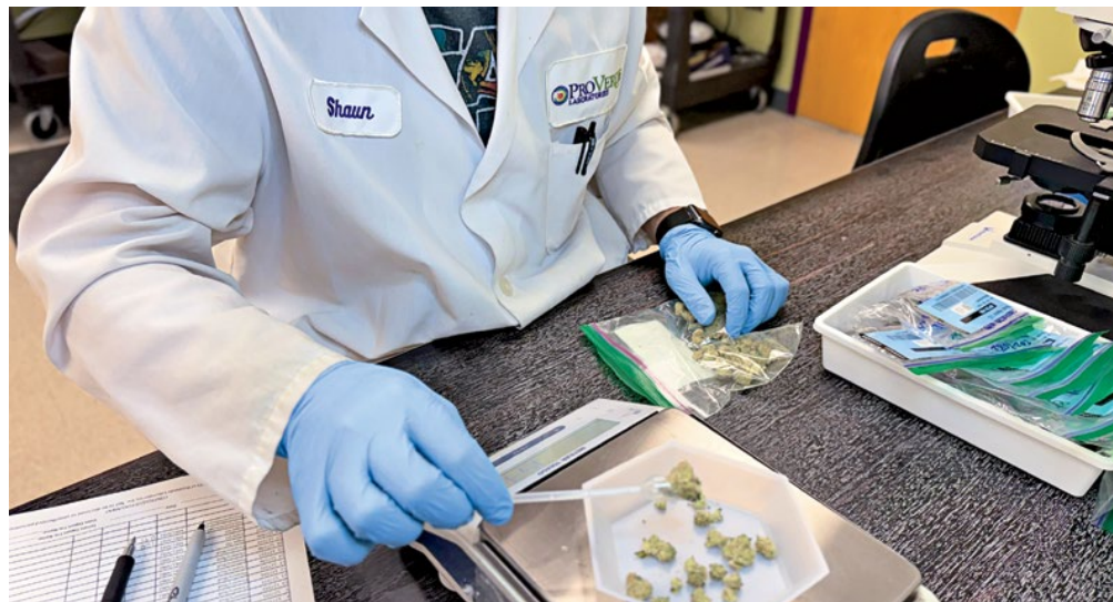
An accurate sample weight is needed to determine the concentrations of cannabinoids in cannabis flower.
