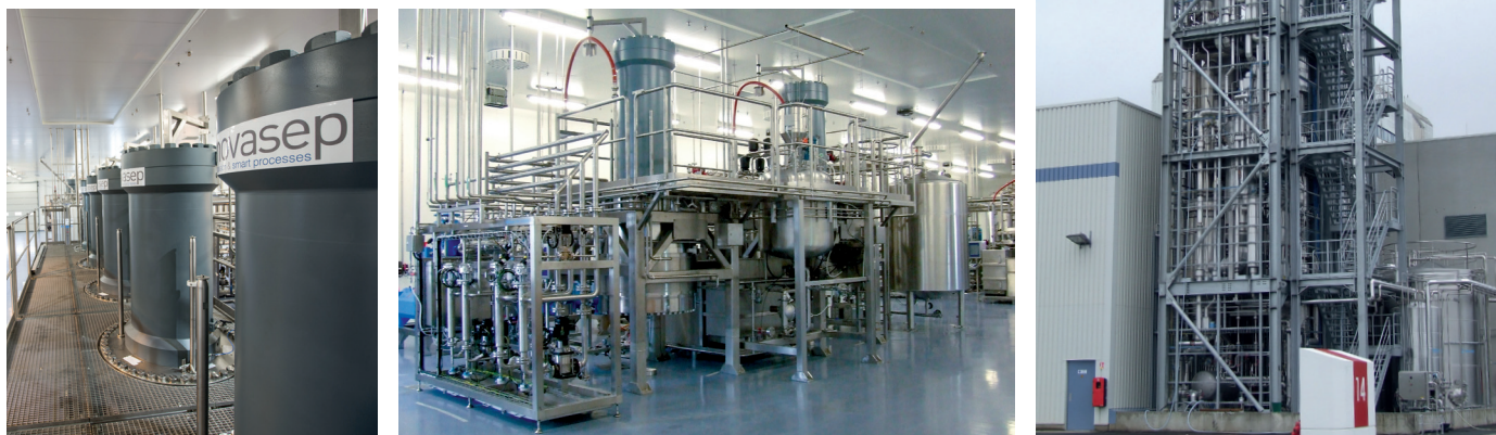
Figure 1. Varicol® (advanced SMB) and Hipersep® with 99.99% solvent recycling for MTon Scale purification of natural extract for pharmaceutical application.
