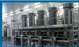
Industrial chromatography unit Varicol (5 columns LC1200) at Novasep Mourenx site (France)
