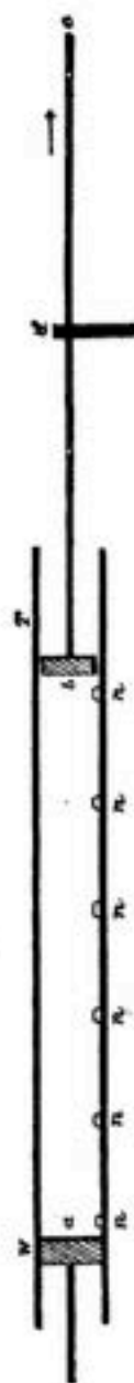
FIG. 66.—Kundt's Dust-Tube Method of determining Velocities in Tubes. WT, wave-tube closed by an adjustable tight piston at a and a loose piston at b . The loose piston is at the end of a glass or metal rod, bc , clamped at its centre, d , and excited by stroking in the direction of the arrow near e ; mnn are the heaps of lycopodium collecting at the nodes.
