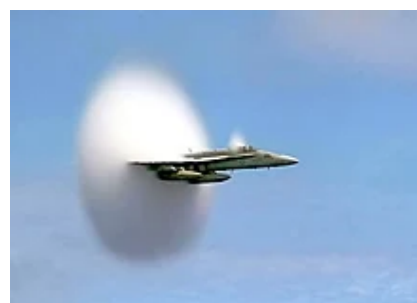
U.S. Navy F/A-18 traveling near the speed of sound. The white halo consists of condensed water droplets formed by the sudden drop in air pressure behind the shock cone around the aircraft (see Prandtl-Glauert singularity). [18]
